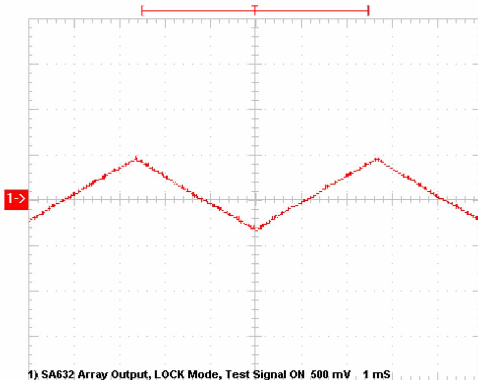
Figure 3-3 Output of the PFL-102 in LOCK mode. The output voltage tracks the applied test signal, which is used to modulate the array.
