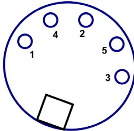
Figure 6-1 Pin assignments for the DIN 5-pin power connector on the rear panel of the PCI-100.
