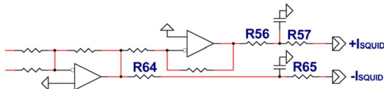
Figure 5-7 SQUID bias circuit schematic. The default value for R56, R57, R64, and R65 is 2.49 k $\Omega$ .
