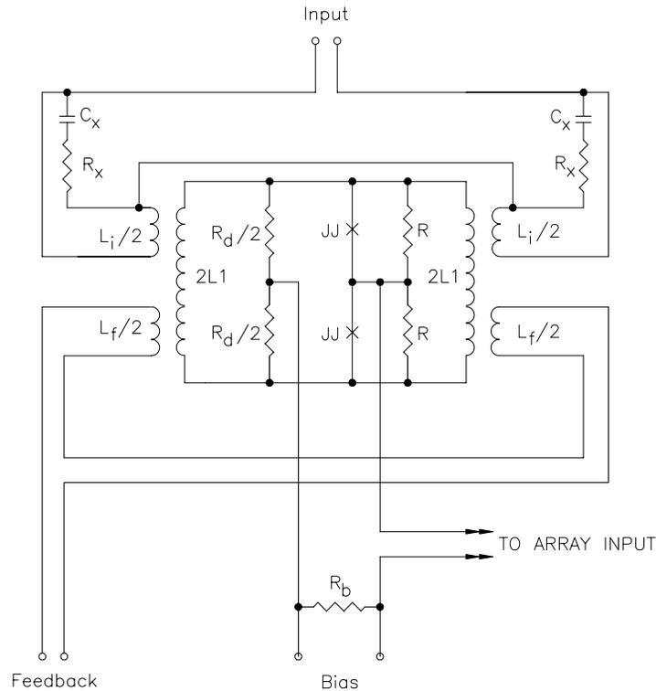
Figure 3-6 Schematic diagram of the input SQUID stage of STAR Cryoelectronics' SA1xx/SA6xx series SQUID amplifiers.
