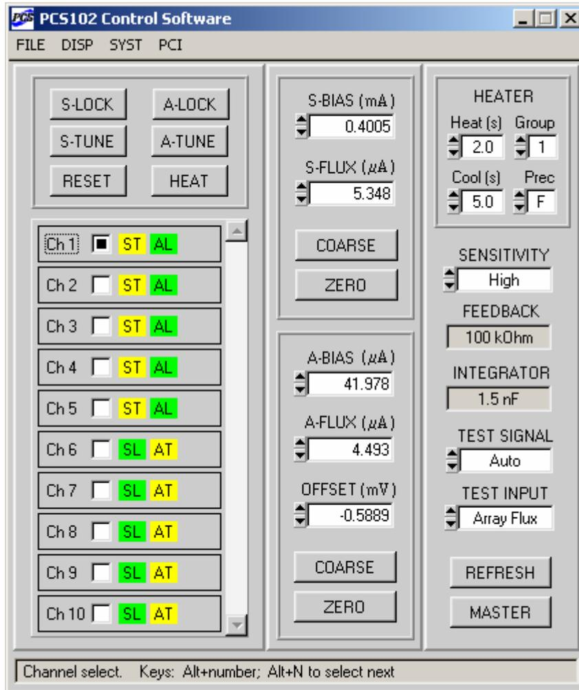
Figure 4-1 The Main panel for 10-channel operation. Channel 1 is the selected channel. All settings displayed on the right correspond to this channel. The first five channels have the input SQUIDS in the TUNE mode (“ST”), and the output arrays in the LOCK mode (“AL”). For the next five channels, the SQUIDS are locked (“SL”), with the arrays in the TUNE mode (“AT”).
