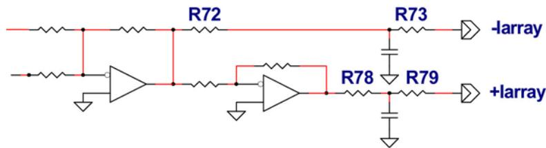
Figure 5-6 Array bias circuit schematic. The default value for R72, R73, R78, and R79 is 49.9 k $\Omega$ .
