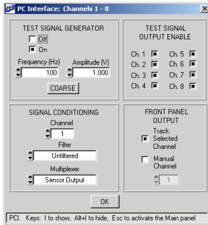
Figure 4-3 PCI panel for channels 1 to 8.
