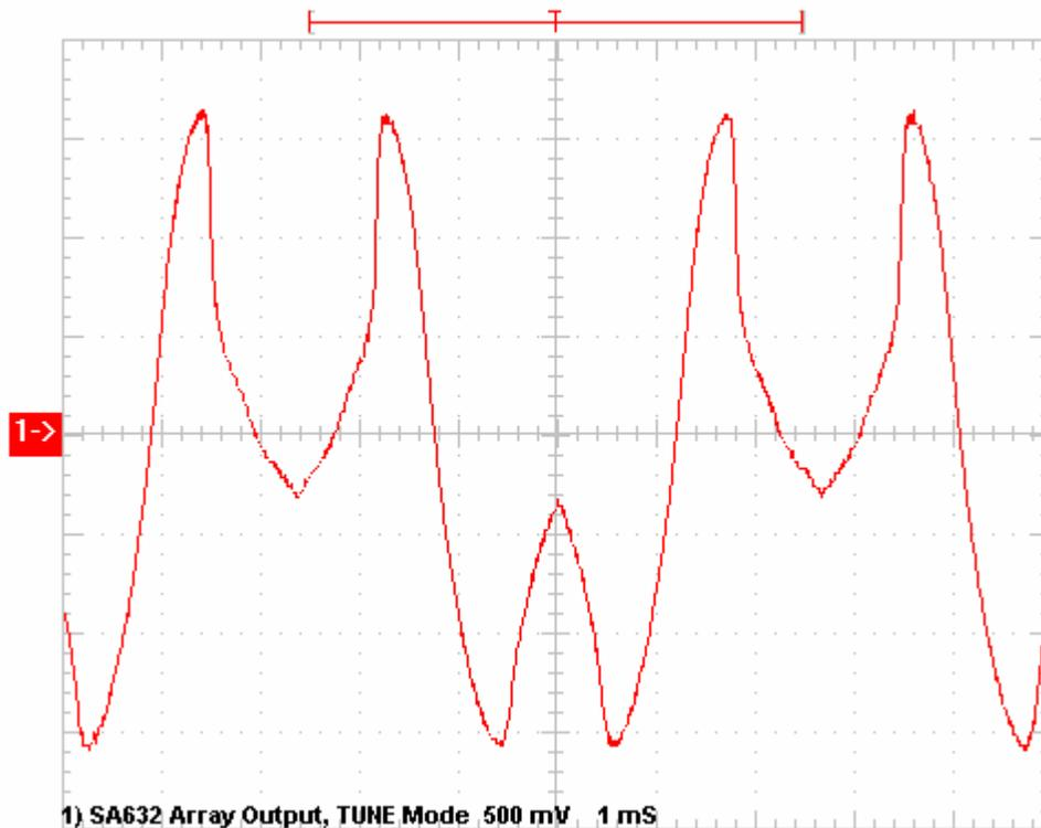
Figure 3-2 Time trace of the PFL-102 output with the array in TUNE mode. A test signal with peak-to-peak magnitude corresponding to  $1 \Phi_0$  is used to modulate the array.
