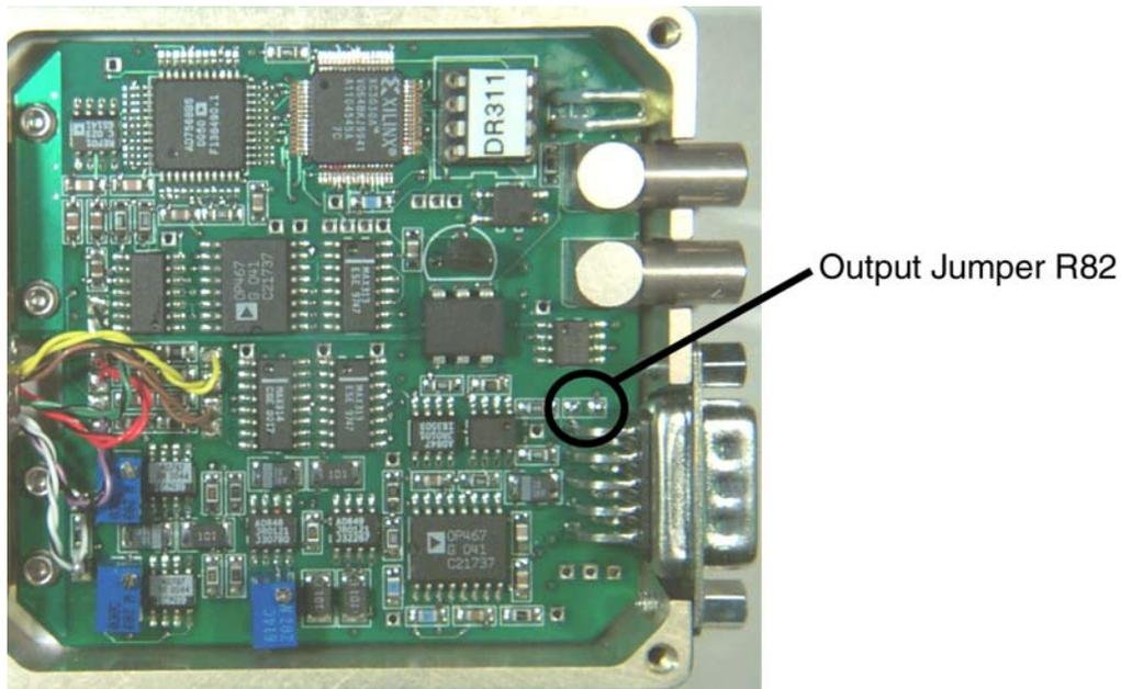
Figure 5-2 Location of the jumper pads to reconfigure the PFL-102 to enable front panel output at the PCI-100 or PCI-1000 interfaces.
