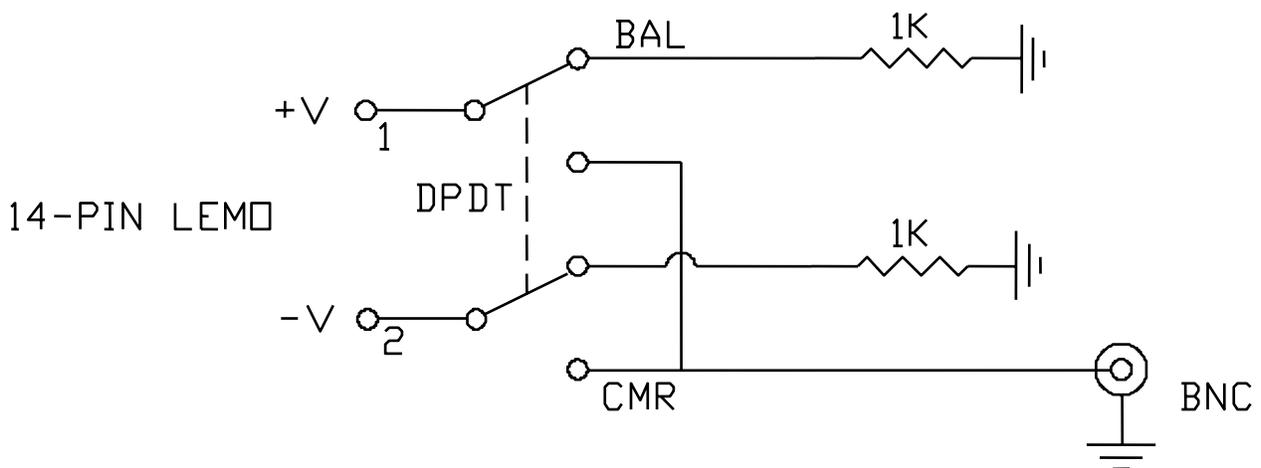
Figure 5-3 Test box schematic used to adjust the preamplifier balance and common mode rejection.
