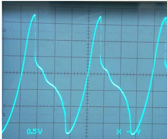
Figure 3-4 Output  $V-\Phi$  characteristic of the array in X-Y mode. The output voltage of the PFL-102 is plotted versus the test signal voltage. Since the PFL voltage gain is 5040, the vertical scale is 0.198 mV/div. The horizontal scale is 2  $\mu$ A/div.
