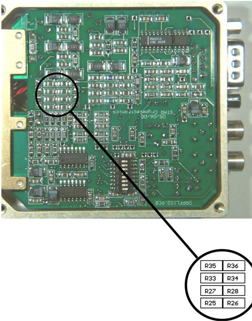
Figure 5-10 Locations of the resistors to set the maximum SQUID and array flux bias current ranges.
