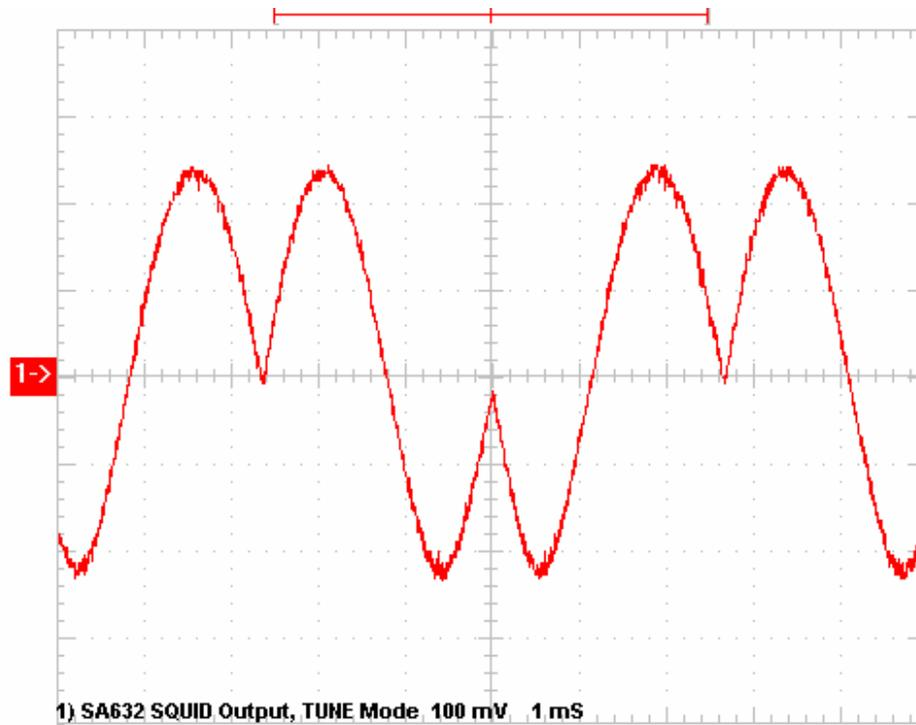
Figure 3-7 Time trace of the PFL-102 output with the array locked and input SQUID in TUNE mode. A test signal with peak-to-peak magnitude corresponding to  $1 \Phi_0$  is used to modulate the input SQUID.
