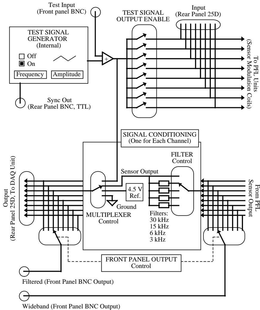
Figure 4-4 Block diagram for the PCI-1000 Interface unit, showing basic signal routing and relationships to the PCI panel software features. Note that this is a relational diagram only. Some features such as buffers, etc., have been omitted for clarity, and wired connections cannot always be interpreted literally.
